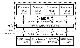
Figure 2. Shared secondary cache multiprocessor.
